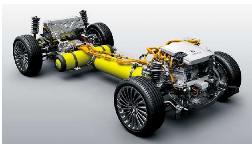
Figura 10 - Toyota Mirai powertrain
