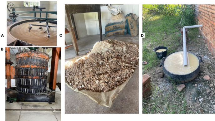
Flour mill: (A) flour production during toasting; (B) cassava pressing to obtain manipueira; (C) flour production residues – cassava peels; (D) flour production residues – manipueira Source: courtesy photo
