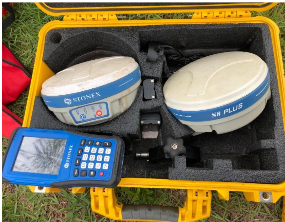
Figura 6 – STONEX S8 plus – RTK.
