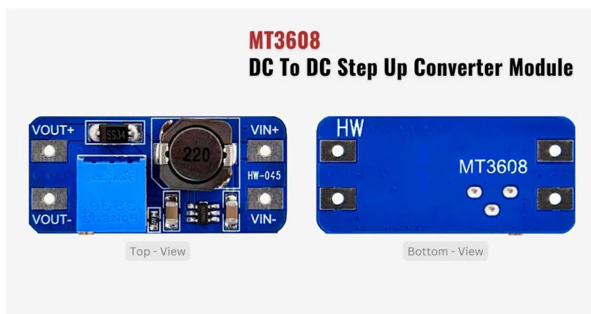
Figura 9 – MT3608 DC To DC Step Up Converter Module. Fonte: (Electrothinks, 2023).
